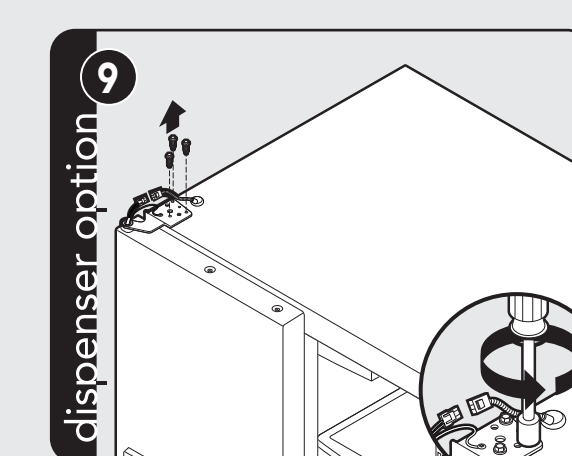
Unscrew 5/16" hex head screws from left top hinge. Retain all screws for later use.
